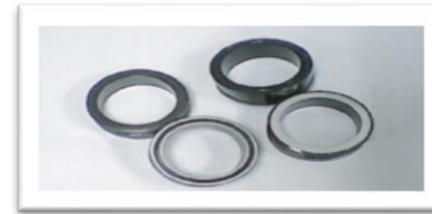
Valve Seat-after Grinding
