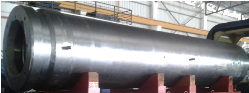
DIA 31" X 144" LG EDM PROCESS AT ID
