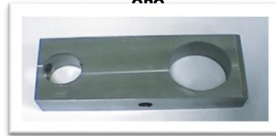
Valve Gate without Nitriding
